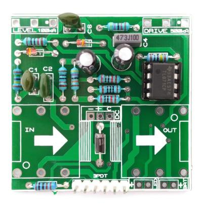
Solder the capacitors and transistors. If you have troubles reading the values, check out our <u>"Reading Part Values"</u> tutorial. Pay attention to the orientation, as well as to the polarity for electrolytic capacitors.
