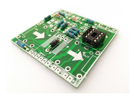
First of all place the IC sockets (without the ICs). Pay attention to the orientation! The small notch in the socket should be oriented as indicated in the PCB.
